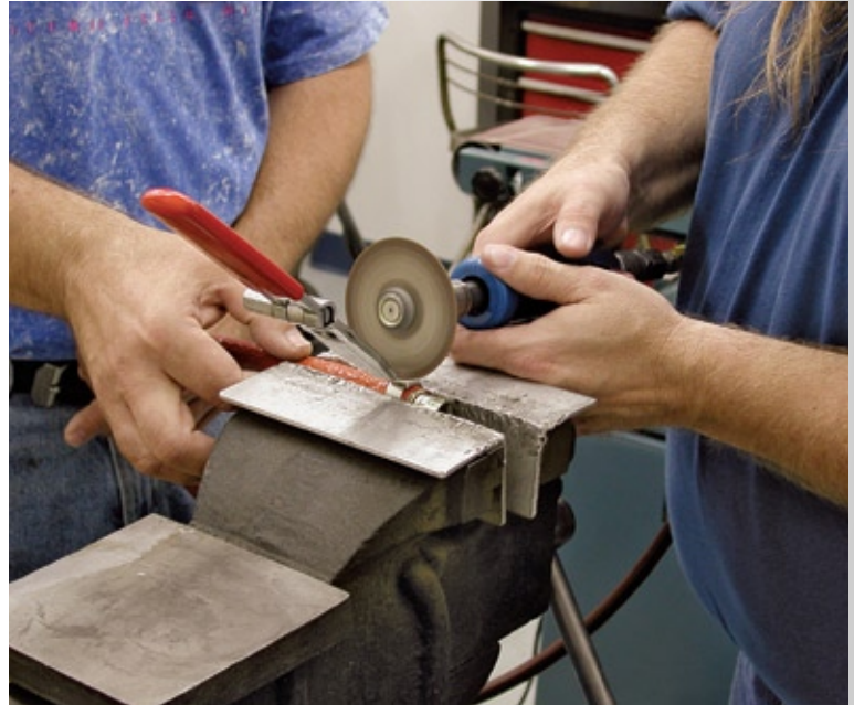
RIGHT BOTTOM: Trimming to size the firesleeve locking band.
