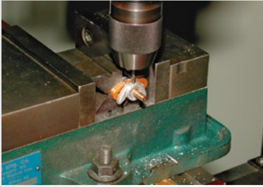
TOP LEFT: Milling the hole for the locking roll pin
